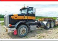
**1989 Peterbilt 378**, day cab, Caterpillar 3406 B ATA, Eaton 13 spd., Peterbilt 4 bag air ride susp., Eaton rear ends, 2 line wet kit, single 100 gal. fuel tank, single exhaust, 24.5 tires, (10) alum. wheels, VIN 1XPFDB9X4KN276437
