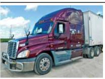
2010 Freightliner Cascadia, 70" standup sleeper, DD15, 475 hp, Eaton FRO-16210C Meritor 40K rear ends, 3.31 ratio, diff. lock, airliner air ride suspension, dual 120 gal. alum. uel tanks, power windows, locks, mirrors, dual air ride seats, air slide 5th wheel, 22.5 LP tires, (6) alum. wheels, VIN 1FUJGLDROASAS9607
