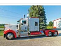
2005 Kenworth W900L, flat top sleeper, 72" aerodyne, C15 Acert Cat 550 hp, twin turbo, Eaton 13 spd., Eaton rear ends 3.36 ratio, AG200 8 bag susp. w/ updated swing arms, dual 15" air cleaners, dual 8" straight pipes, dual step boxes, dual 120 gal. fuel tanks, 18" frame mount step box, stainless steel light bar & lights, stainless air box
