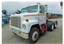
1978 International, day cab, Cummins 290 hp., Eaton 9 or 10 speed, Rockwell SQ100, 3.73 Ratio, Reyco spring suspension, air slide 5th wheel, dual 100 gal. steel step tank, 22.5LP tires, (2) alum, (8) steel, VIN DA227HHA21125 (DOES NOT RUN)
