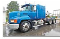
**1994 Mack CH600**, 40" sit down sleeper, Mack E6, 350 hp, Eaton Super 10, Mack air ride susp., air slide 5th wheel, dual 120 gal. fuel tanks, tilt, AC, cruise control, dual air ride seats, 11R 24.5 tires, (6) alum. wheels VIN 1M1AA13Y4RW039192
