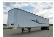
1996 Trailmobile, dry van, 53'x13'6" translucent roof, 110" door opening, plywood lined, alum. scuff plate, threshold plate, 2 spd. landing gear, sliding tandem, air ride susp., 22.5 LP tires, steel budd wheels, VIN 1PT01JAH3T9008181
